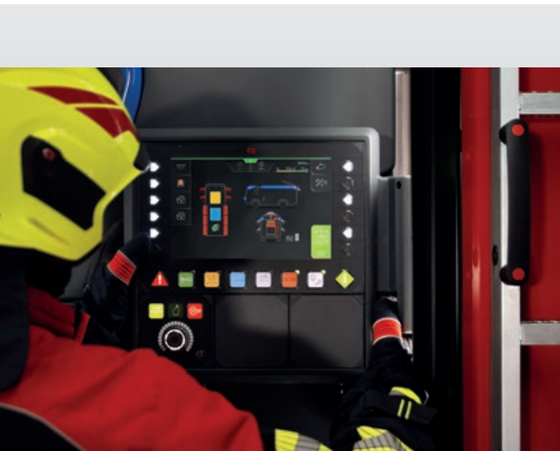
Height-adjustable RBC LCS 10" display with DIGIPOT in the rear.
