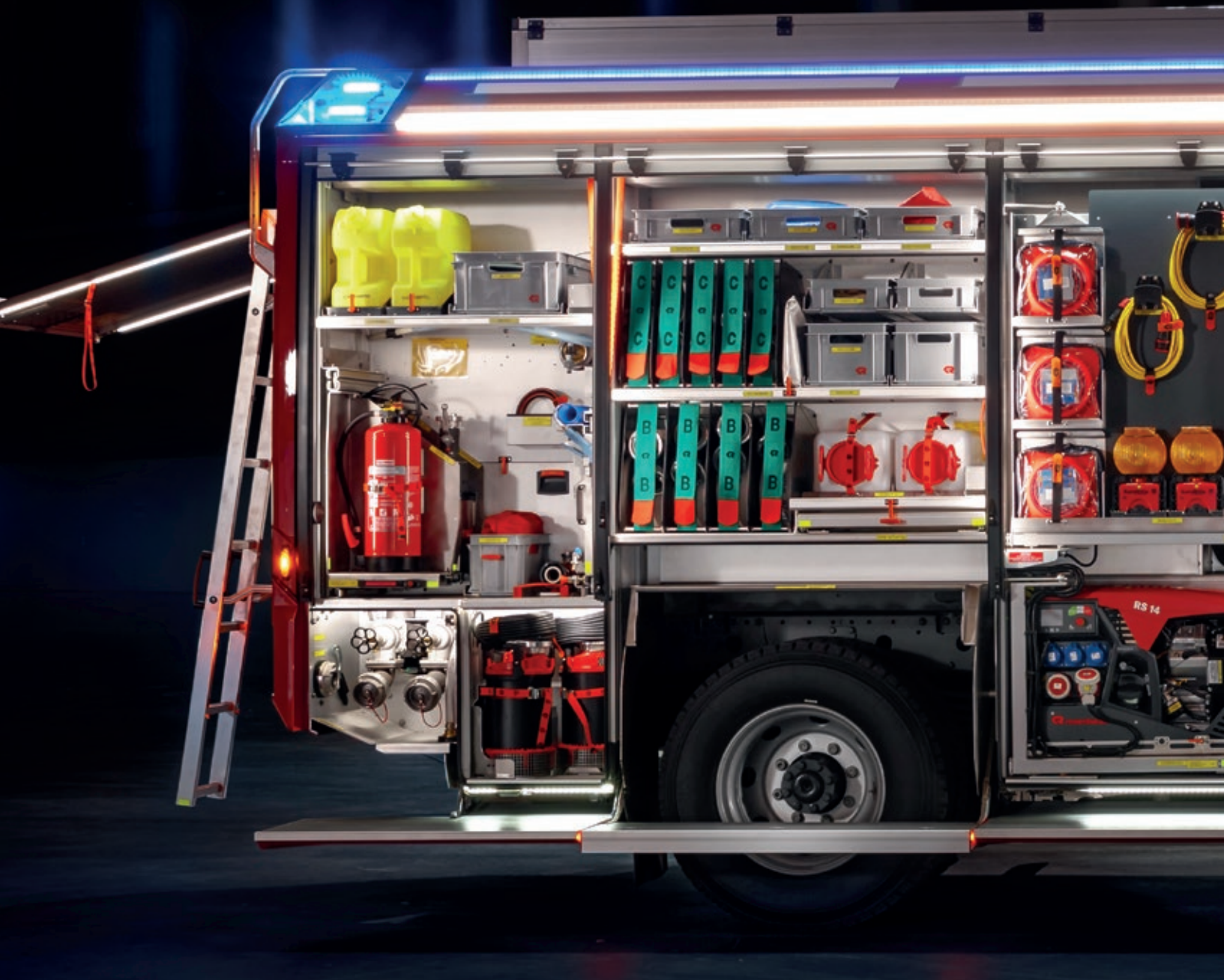
Scene and equipment compartment lighting as well as floor contour lighting.
